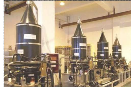
Lower Hybrid Current Drive (LHCD) with Thales klystrons manufactured in Vélizy (France)
