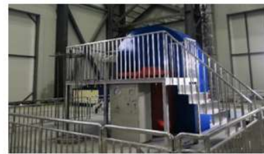
φ500×1500 Hot isostatic pressing system
