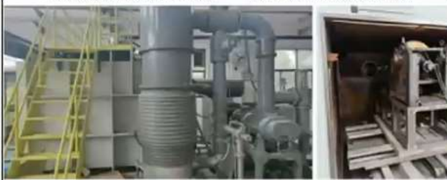
THDW-20 Electron beam welding equipment (3m×2m×2m, 85kV/20kW)
