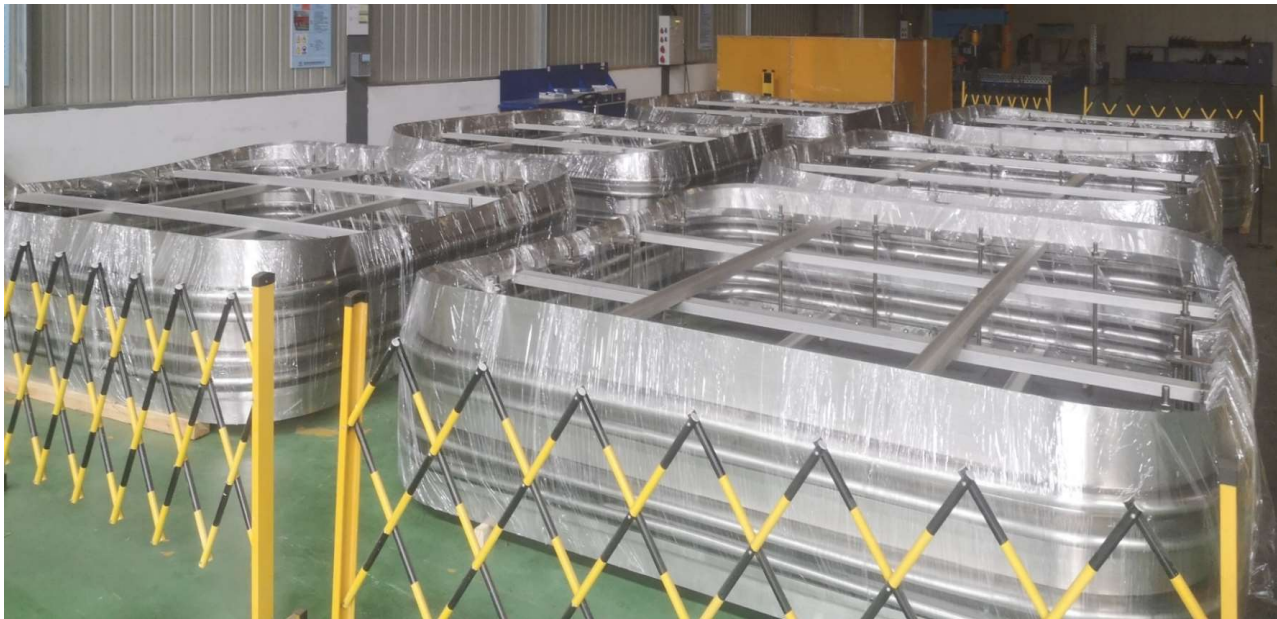
Large cross section (3m*4m) rectangular bellows
