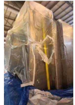
Tested at Site for the global Helium Leak requirement of 10e-7 mbar l/s (2025)
