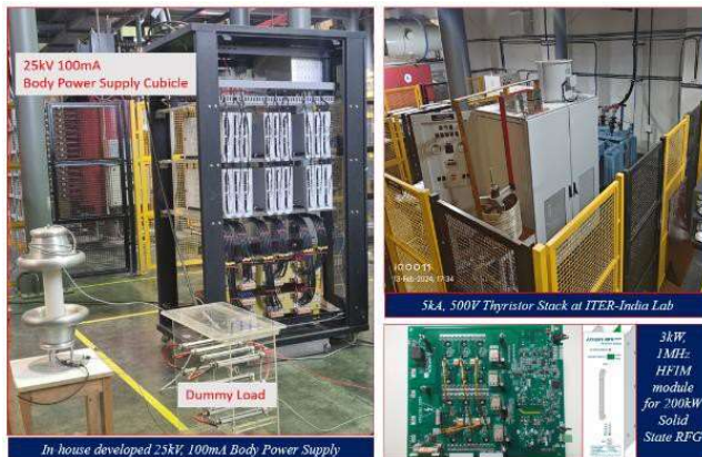
25kV, 100mA Body power supply developed for Gyrotron using a new control topology
