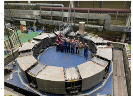
PF1: D=9\text{ m} , 160 tons
