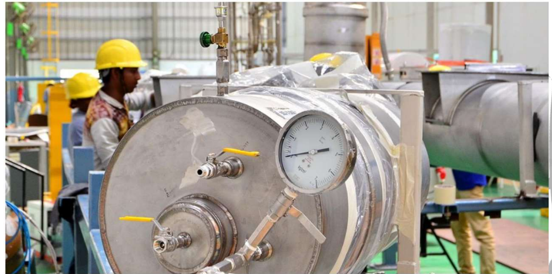
Multi-metre-long cryolines during fabrication at M/G INOXCVA, Vadodara, in 2019
