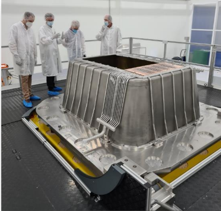
Grounded grid on the 15tons 90° tilting assembly structure
