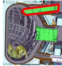
Upper Port Plugs (UPP) ~ 25 tons
