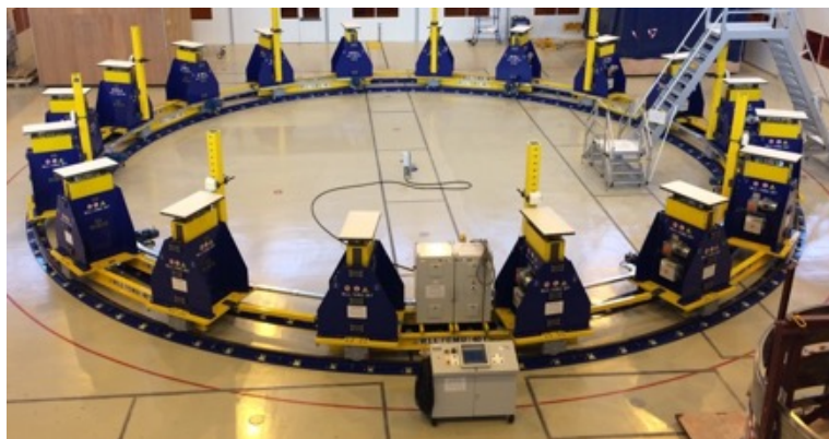
PF coil manufacturing tools
