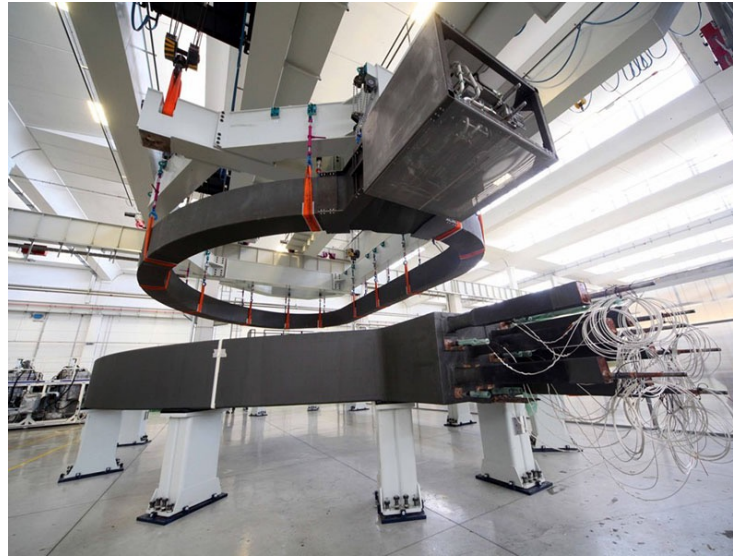
ITER TF coil winding pack
