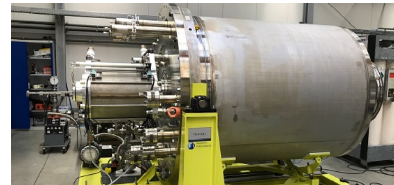
Cryogenic pumps for ITER
