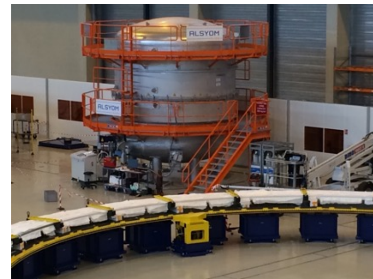
Test cryostat and PF coils manufacturing tools
