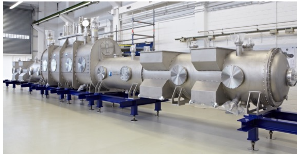
KATRIN experiment: Windowless Gaseous Tritium Source (annual tritium throughput app. 10 kg in a closed loop)
