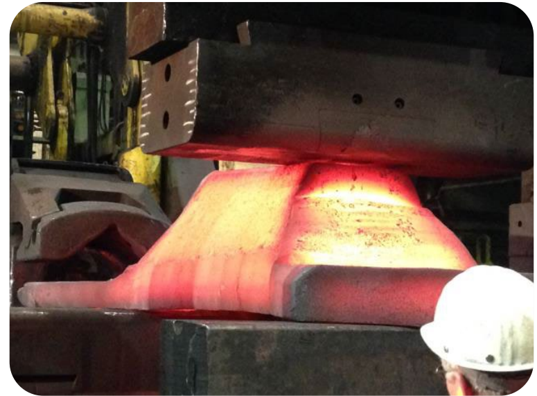
ITER TF Coil Structure – Wing Forging Total of 68 Pieces
