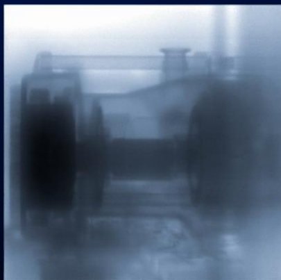
Laser-driven image: through 3cm of aluminum, <1ns exposure
